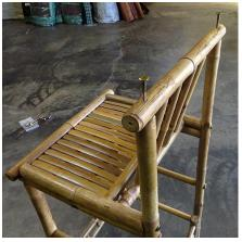
Then 2 holes on the back the go through the back of the Side pieces into the Seat piece. And finally 2 the go up from the underside of the Side piece into the underside of the Seat piece.
