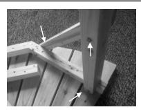
2. Setup the other leg as shown on the previous step using the same bolts and pieces.
