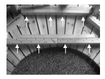
3. Set up the two seat pieces as shown above and using the 23" straight slabs match the four corresponding holes and secure the midsection of the bench using 3 <sup>1/4</sup> " bolts along the bottom while the 23" piece used along the top will use the 3  $^{1/4"}$  bolts at the far right and left end holes only.
