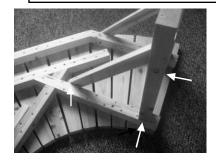
1. Setting one seat panel, match one of the wood legs to the inside portion of the bench. Using a 2  $^{3/4"}$ bolt attach the leg to the bench. Then setup one of the angle supports and match one end to the leg as shown above using a 3  $^{1/2"}$  bolt while using a 3  $^{1/4"}$  bolt to secure the other end directly onto the bench.
